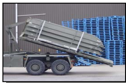
Unloading the pontoon boats ready for shipping
