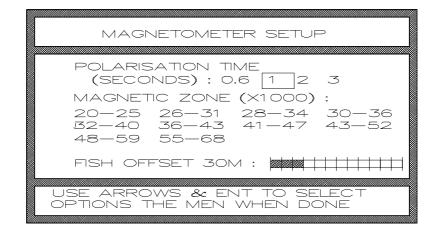
NB. The above diagram shows the existing options within the SETUP MENU, however the settings related to these MAGNETIC ZONE options have been further optimised as per the diagram and conversion list below: -
