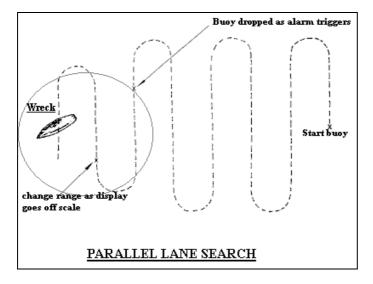
speculative basis, or where the position of a wreck is very approximate (**PA**), it is also a more precise way of covering a preplanned area of seabed as a square or rectangular shape.
