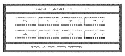
The above display confirms the extended 256Kbyte RAM configuration is fitted; each position is occupied and is equivalent to 32Kbyte. In the case of the AX2000 PES & PET this equates to 8 x 32 i.e. 256Kbyte, this is the maximum capability, and allows a data-logging storage time of approximately 10hrs duration.
