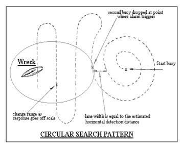
The circular search pattern is particularly suited when a graphical plotting navigator can be used in conjunction with the AX2000 magnetometer.
