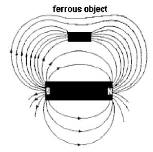
THE MAGNETIC ANOMALY OF A FERROUS OBJECT IN A UNIFORM MAGNETIC FIELD
