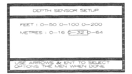
The above menu selection allows for the units displayed to be selected as feet or metres, this is effected by highlighting the required range in the relevant units and pressing the **ENT** key followed by the **MEN** key to return to the MAGNETOMETER MODE MENU.
