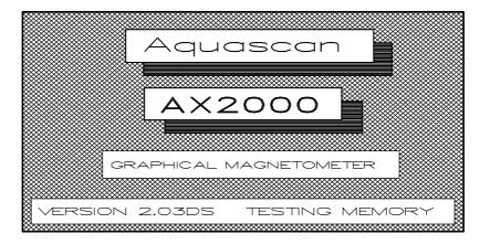
This screen will be present for approximately 10-15 sec's. During this time the AX2000 will perform its memory test. The words "TESTING MEMORY" will appear in the lower half of the screen and the sounder will emit a rapid burst of clicks. The version of software fitted to the AX2000 is also indicated. When the memory test has been successfully completed, a new screen will be display memory configuration installed e.g. 256Kbyte.
