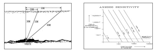
By taking the maximum sensing distance for a given target and producing a simple scale diagram - the optimum search lane width can be derived. The procedure is as follows: -
