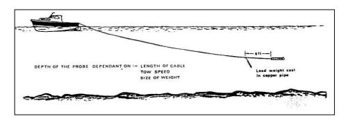
In cases where the object to be detected is at a depth that would not allow positive detection with the tow-fish at the surface, requires that the tow-fish be deployed at a height above bottom that would guarantee a response within the search parameters employed. The use of a lead ballast weight close to the tow-fish, is a simple but effective method of achieving increased tow-fish depth for a given speed.
