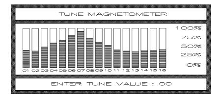
Once the TUNE MAGNETOMETER mode is selected the AX2000 automatically scans through the available tuning steps, measuring the signal strength for each step.
