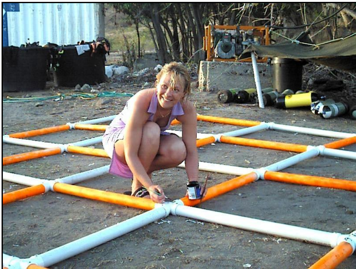
Illustration 10: Painting the alphanumeric numbers on the cross pieces which will identify the individual squares (© ADMAT Archives).
