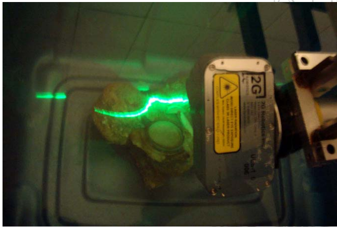
Photograph 14: The green laser scanning the concretion underwater (© ADMAT).
