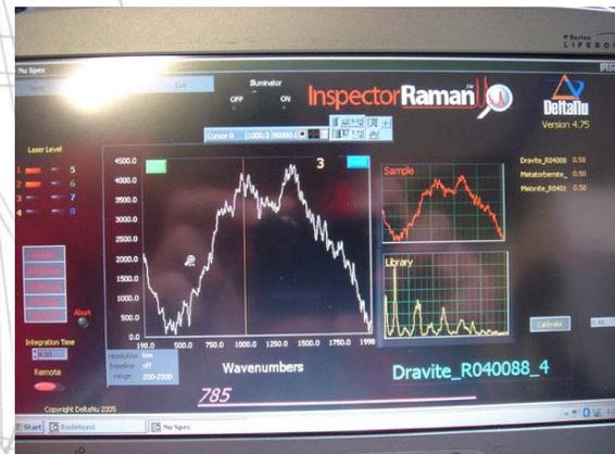
Photograph 19: The computer screen showing the RAMAN test results from the analysis of a medicine phial bottle from *Le Casimir* (© ADMAT - Spooner).
